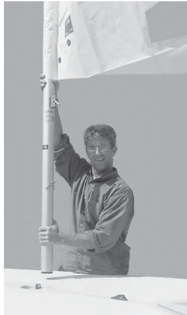
figure 30a: Stepping the Mast
